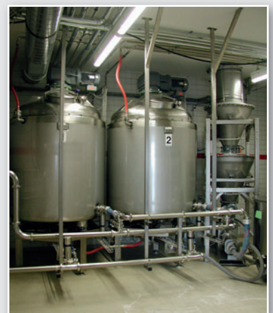
Predough plant with external mixing station for dough yield
